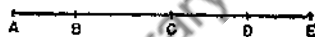
FIG. 4. The line AE and its four segments have been measured. The sum of the adjusted segments must equal the adjusted over-all length.
